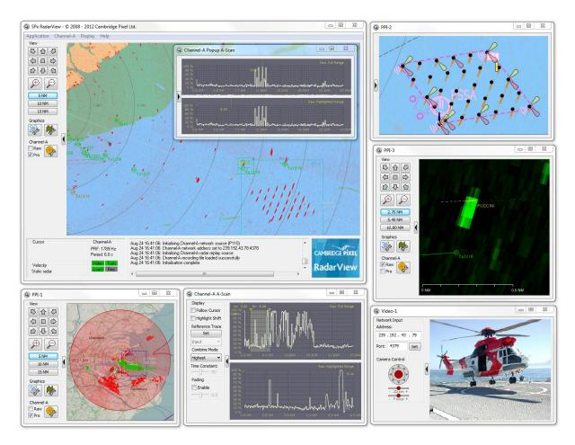
Figure 1 - The SPx software library may be used to build complex radar processing and display applications. The open framework software architecture means that library SPx modules can be mixed and matched with custom application and GUI software.
