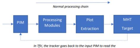
In TJV, the tracker goes back to the input PIM to read the raw radar video. This occurs when the TJV mode is enabled and no plot is received through the normal processing chain
