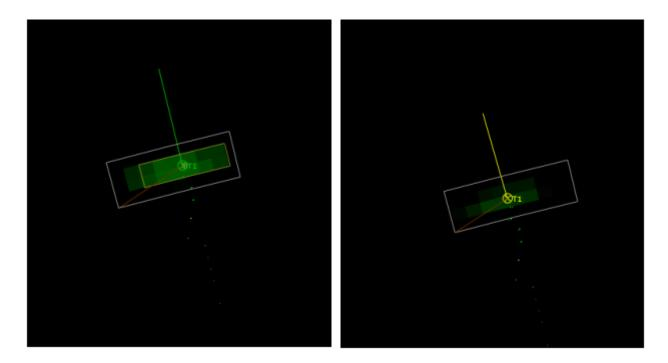
One application of TfV is to extend the time of tracking of a target by permitting updates after plots are lost. However, the success of this depends on there being some low-level, intermittent target video present. If there is no video present then TfV will have no affect and the track will coast as normal. In this situation there is nothing lost by enabling TfV.
