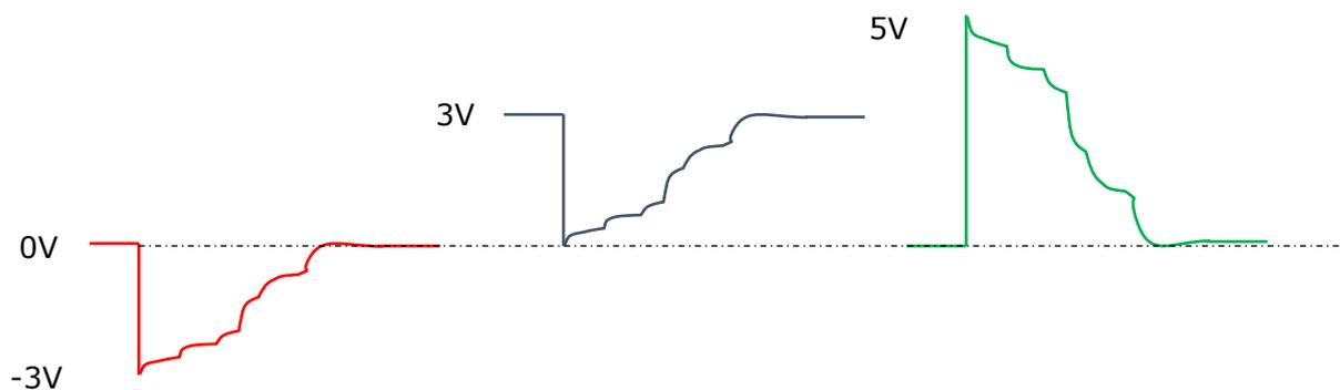
1. The video signal coming from the radar ranges from 0V (no signal / black level) to -3V peak.
