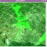
In the first stage, scan converted radar video is inserted into the application. The significant point of this first stage is that the graphics application is completely unchanged – no code changes, no re-linking. It's exactly the same graphics application that now has radar video presented inside it. The radar video processing is done in a separate software process, which captures the video data, processes it, scan converts it
