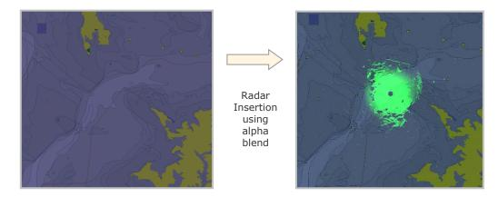
The window on the left shows the application graphics. After insertion, the radar video is combined with the graphics so that the output is a blended version of the two images. The brightness and emphasis of the radar video can be controlled in the blending process. As before, no code in the graphics application has been changed to implement the radar insertion.
