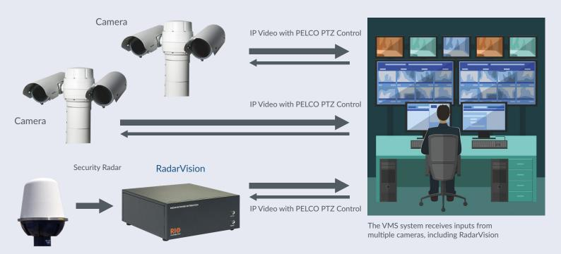
RadarVision sits between the radar and the display system. It receives radar data (video, plots or tracks) and converts the data into an image with maps and symbols which is then sent to the video display system.
