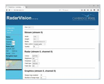
RadarVision adds high fidelity radar imagery into a security display, allowing camera and radar to be viewed together. The high-resolution radar image may be zoomed and panned using an on-screen or physical joystick.
