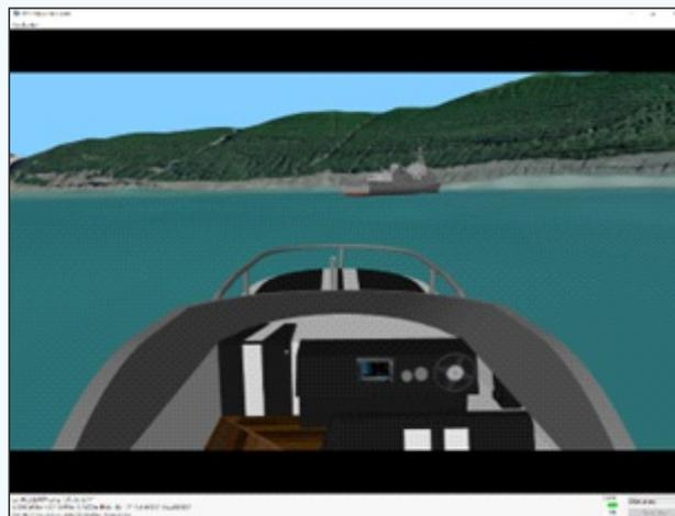
Targets moving in the scenario have properties including a 3D model that is used to render the target for the current camera view.
