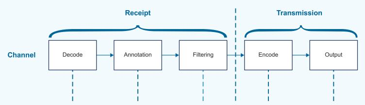
Schematic diagram showing the different processing stages for a single channel. In addition to each channel acting as a totally separate process it is also possible to duplicate the output from any stage of another channel in order to create a new one. Each subsequent stage can then be performed differently on the new channel as required.
