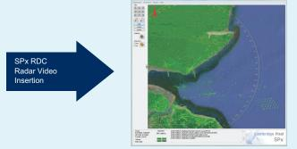
Client application PPI window after RDC radar video insertion
