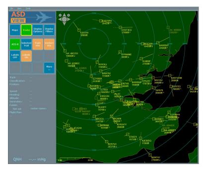
ASD-View is Cambridge Pixel's PC-based display application for ADS-B receivers. It is a complete ready-to-run Windows application for the display of target positions and associated information.
