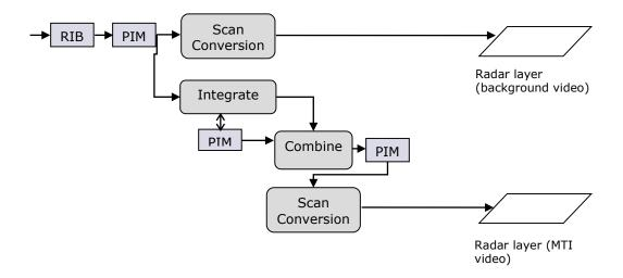
The *Integrate* process takes input from the main input PIM and derives an Integration PIM to hold the integrated data.
