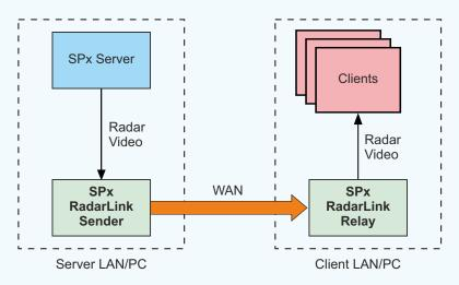
RadarLink addresses the problems of unreliable or low data rate connections using three approaches:
