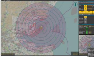
USVx is a client-side application, available as an executable or development package, which provides a remote display of radar video, tracks, AIS and radar status.
