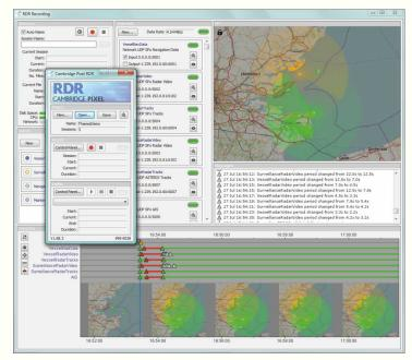
RDR is a Windows-based multi-channel, multi-format data recorder. It can be used to capture all sensor data during trials for replay and analysis.
