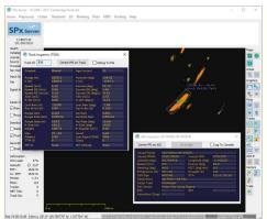
Parameters of the track processing can be used to control the speed of detection, area of interest, track dynamics and filtering. The output of the processing is track reports which may be distributed off the boat using normal communications methods, and/or used by further processing on the boat for fusion or navigation.
