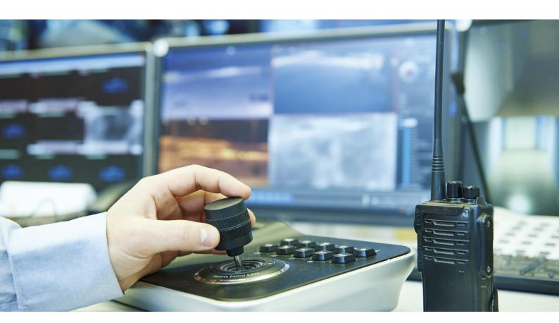
The operator observes an area of interest and uses the VMS's joystick to select it and zoom in for a closer view.
