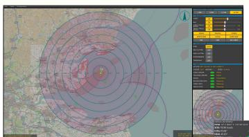
USVx is a client-side application, available as an executable or development package, which provides a remote display of radar video, tracks, AIS and radar status.
