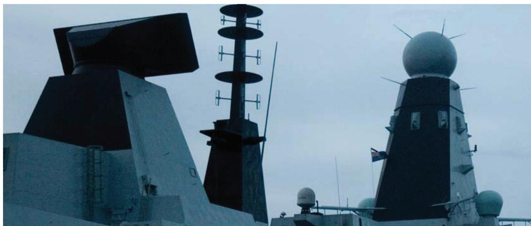
Above: Mission Systems' Long Range Radar and Sampson Multi-function radar are prominently situated on the Type 45 Destroyers such as HMS Daring, pictured here
