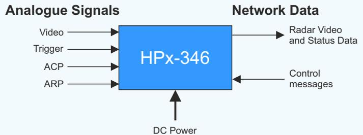
With the HPx-346 unit, an analogue radar video output can quickly and easily be turned into an open network data stream that multiple clients can access.
