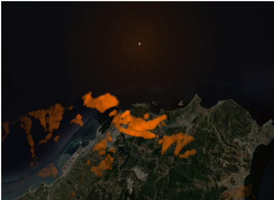
Figure 1: Example of radar misalignment – orange radar video is not well-matched to the physical features shown in the map underlay.
