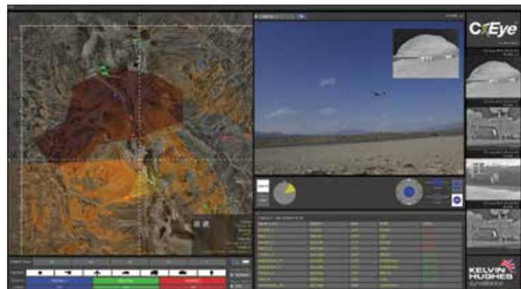
The CxEye application was developed for Kelvin Hughes to provide a visual display of multiple surveillance radars, cameras and target tracks. The software is built using the Secure-X software modules.
