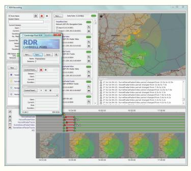
RDR is a Windows-based multi-channel, multi-format data recorder. It can be used to capture all sensor data during trials for replay and analysis.
