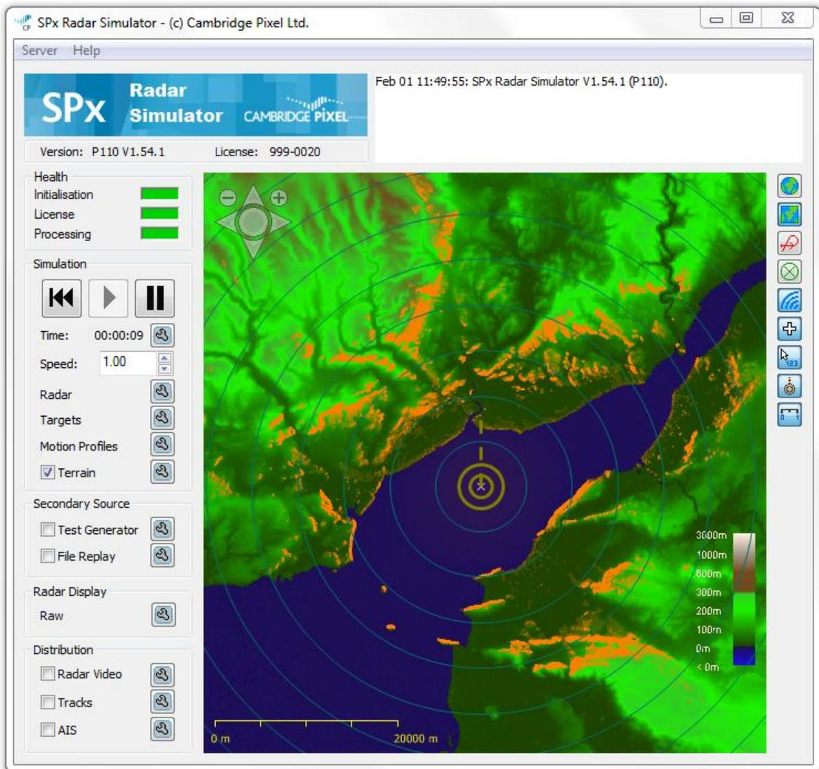
**Figure 2 - SPx Simulator may be used to create simulated radar video, along with related GPS, navigation and track information. The video may be output in Asterix format along with standard TTM track messages and NMEA GPS signals. The display above shows the display of the product.**
