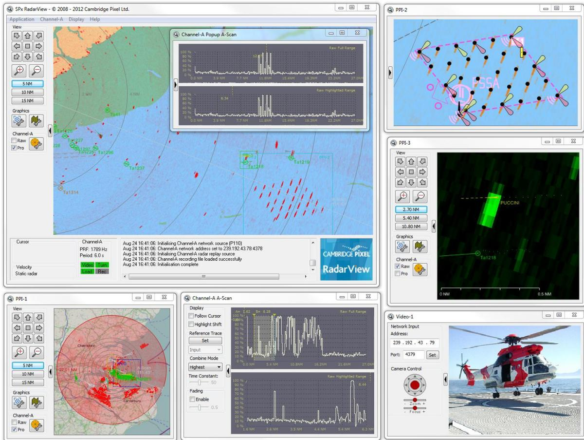
**Figure 1 - The SPx software library may be used to build complex radar processing and display applications. The open framework software architecture means that library SPx modules can be mixed and matched with custom application and GUI software.**
