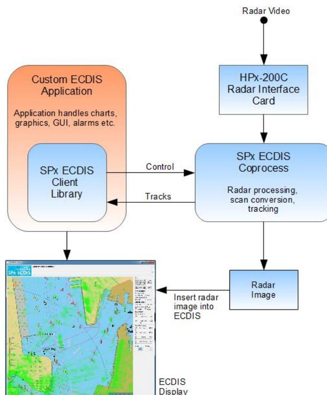
**Figure 3 - Cambridge Pixel's RadarView application is built on the SPx libraries and software scan converter. The software can receive Asterix video from a network and scan convert for display with maps and targets.**
